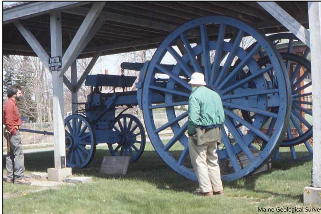
Figure 1. Granite hauling wagon called a galamander.
