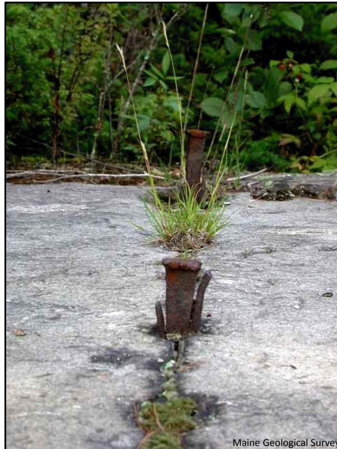
Figure 5. Wedges and feathers in grain of granite from Tayntor Quarry, Hallowell.
