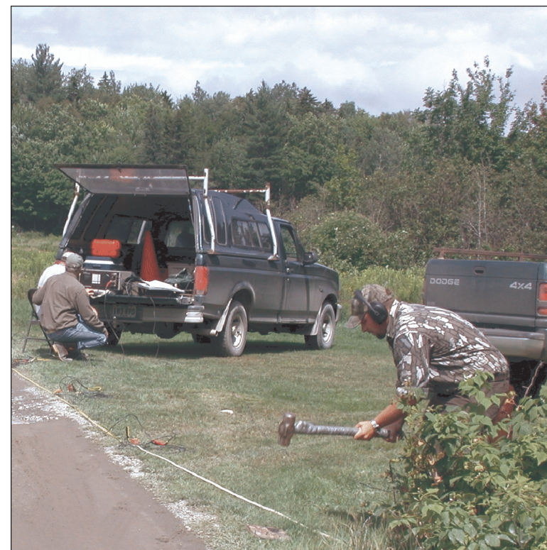
Operating a twelve-channel seismograph, Piscataquis County, Maine.
