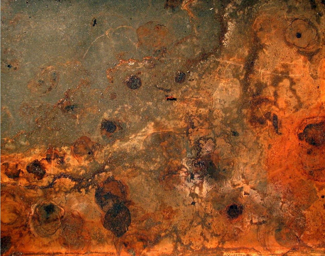
**Iron oxide on a steel baking pan.** Iron oxide, commonly known as rust, is the most familiar example of corrosion. Photo credit: Roger McLassus.
