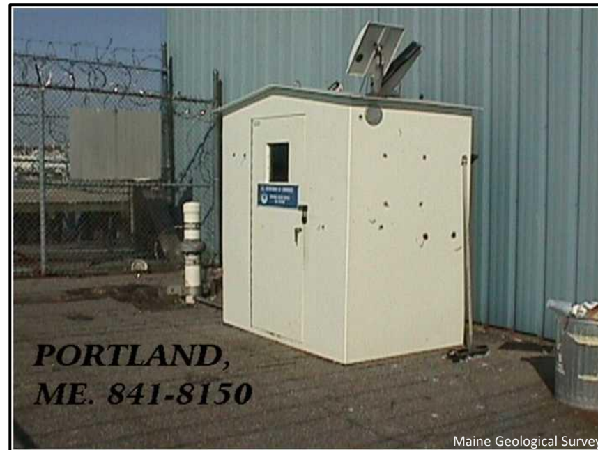
Figure 1. The small white building supports the operation of the Portland tide station. A vertical pipe or "stilling well" that removes the influence of small waves extends down below the pier into the ocean (to the left of the building).
