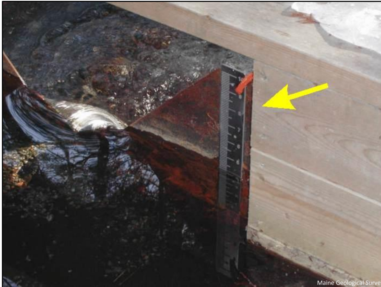
Figure 7. View looking downstream at 90 degree v-notch weir. Note location of staff gauge used for determination of upstream stage for flow correlation.
