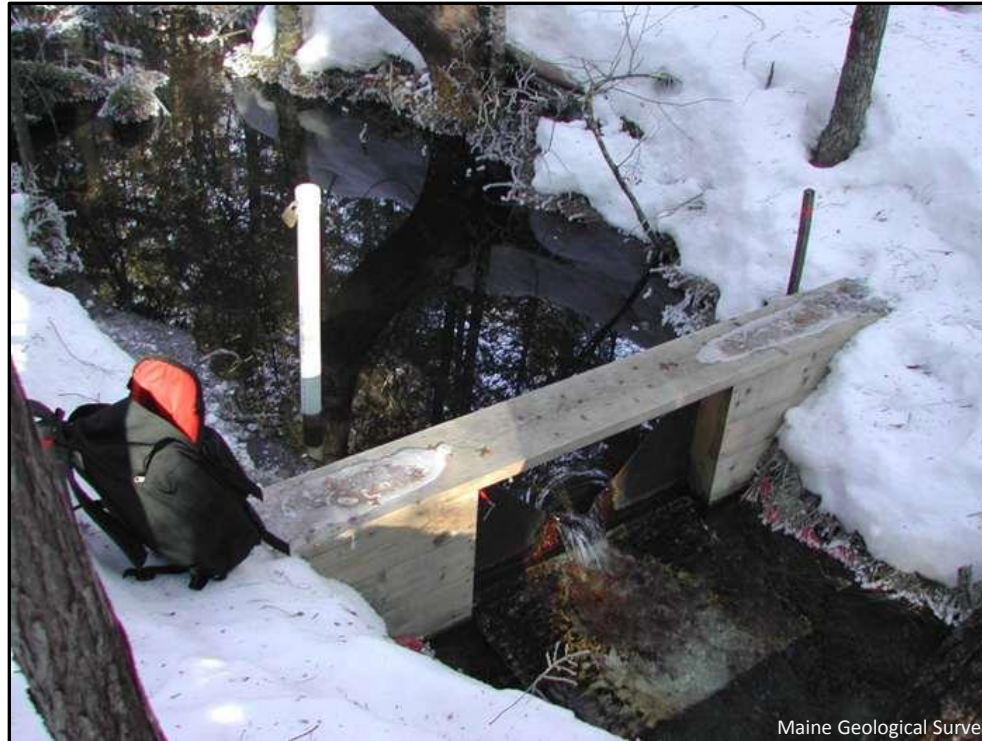
Figure 5. View upstream of 90-degree v-notch weir. Note splash plate downstream to prevent scour. The weir plate is installed by driving it into the stream sediment. For accurate measurement, it is absolutely essential that no or very minimal leakage occurs around the weir.
