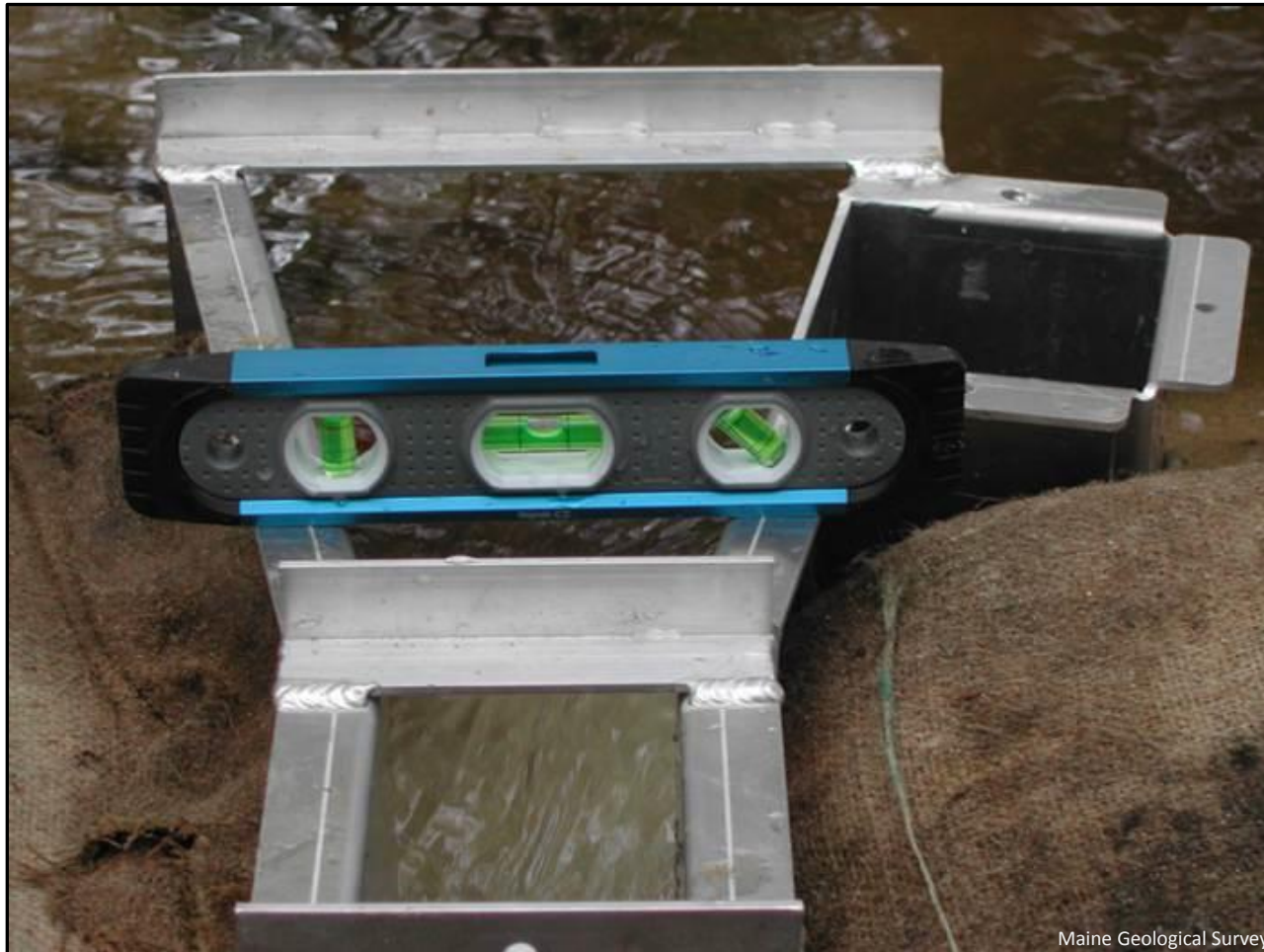
Figure 2. View looking upstream at USGS 3-inch Modified Parshall flume with torpedo level across width. When installing a flume, the unit must be level along the length as well as the width.
