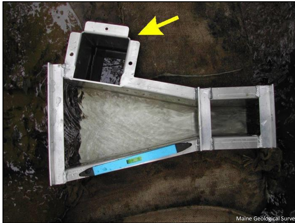
Figure 1. Top view of USGS 3-inch Modified Parshall flume with torpedo level. Note the stilling well where stage level is measured.
