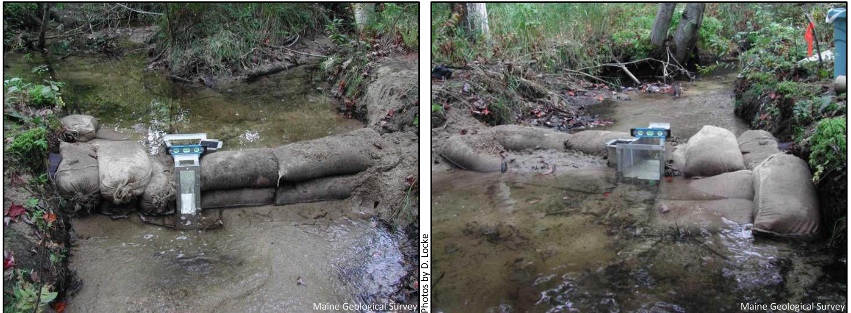
Figure 3. Views of the USGS 3-inch Modified Parshall flume. Note extensive sandbagging to prevent/minimize leakage. (Left) Looking upstream. (Right) Looking downstream.
