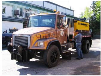
In 2010 MaineDOT purchased an FP5 unit from Bergkamp for Maintenance & Operations' Southern Region. The unit was shipped from Kansas to Maine. The Department provided a truck from their fleet to accommodate the FP5 unit which was installed by MaineDOT personnel.
