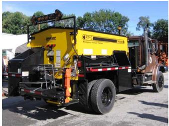
The Bergkamp pothole patcher utilizes flameless (electrical) heat technology to keep the asphalt material at optimum working temperatures. The electrical generator runs off the truck's transmission supplying 240 volts at 1800 rpm. Two 240 volt tube heaters run the length of the hopper with controls to regulate the actual temperature of the asphalt material in the hopper.
