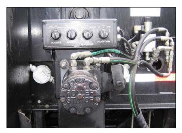
Rear-mounted hydraulic controls are within easy reach of the operator. These controls regulate auger speed (discharge rate) and raising & lowering of the rear-mounted tool platform.
