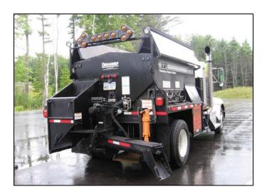
The FP5 is a truck-mounted all-in-one pothole patcher. This particular unit was based on a Kenworth chassis.
