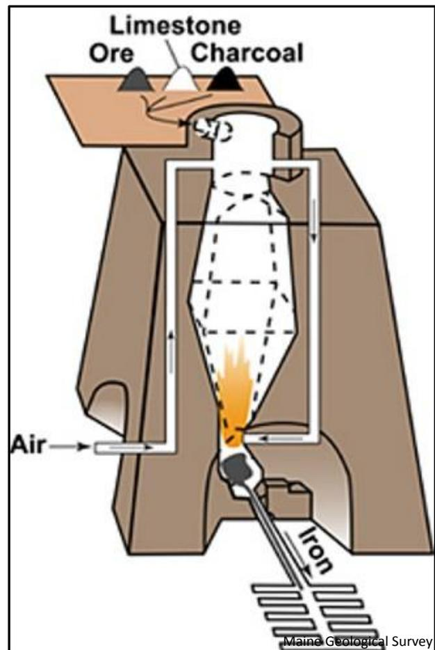
**Figure 6.** Diagram of workings of blast furnace ([from Katahdin Iron Works website](#)).
