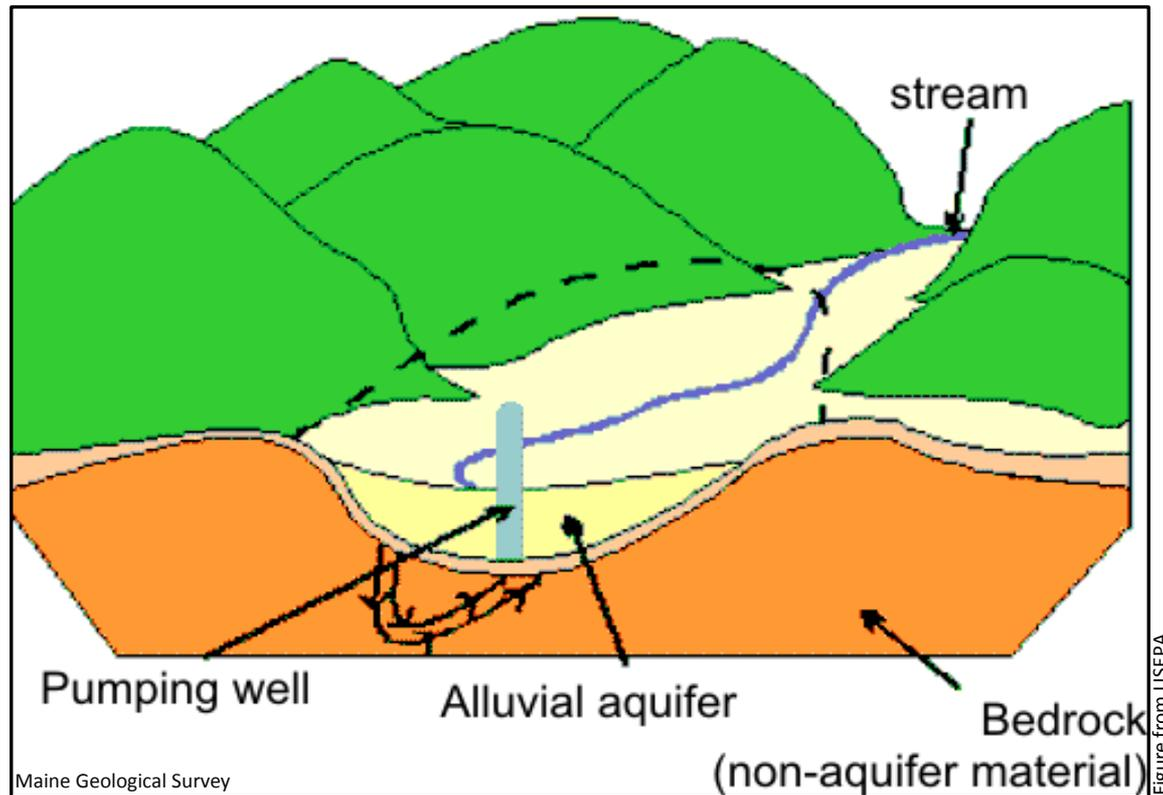
**Figure 2.** This schematic block diagram shows a typical valley fill aquifer in mountainous terrain, like Bingham. The till and bedrock uplands may also provide some water to the well, both through ground water flow and from induced infiltration of stream flow from the uplands
