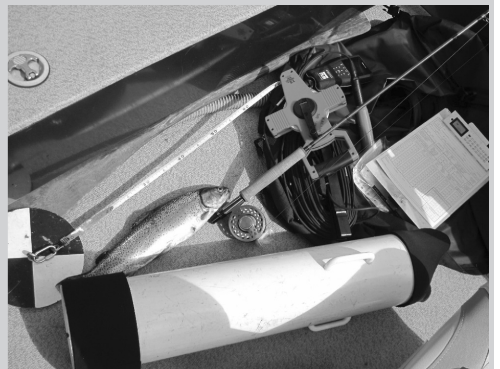
Tools of the trade: WQ Meter, Secchi disk, Aquascope, and nice Rainbow Trout caught by fishing at the right depth in the temperature-oxygen profile.
