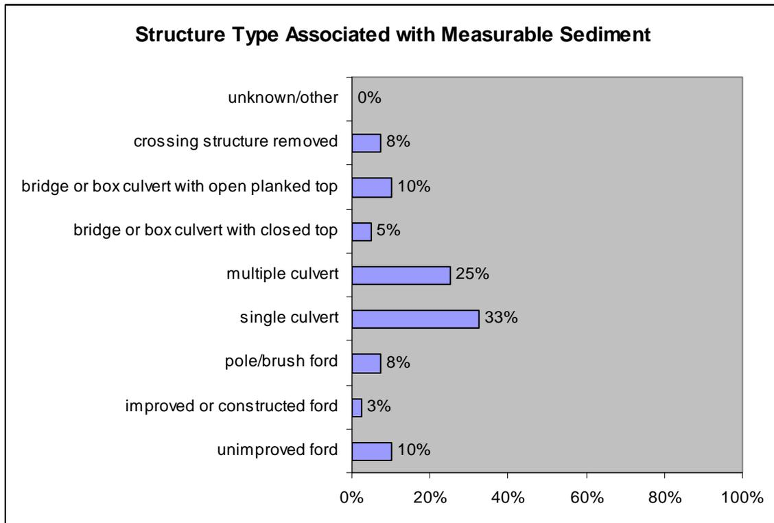
**Figure 13** Structure type associated with measurable sedimentation (n=40).
