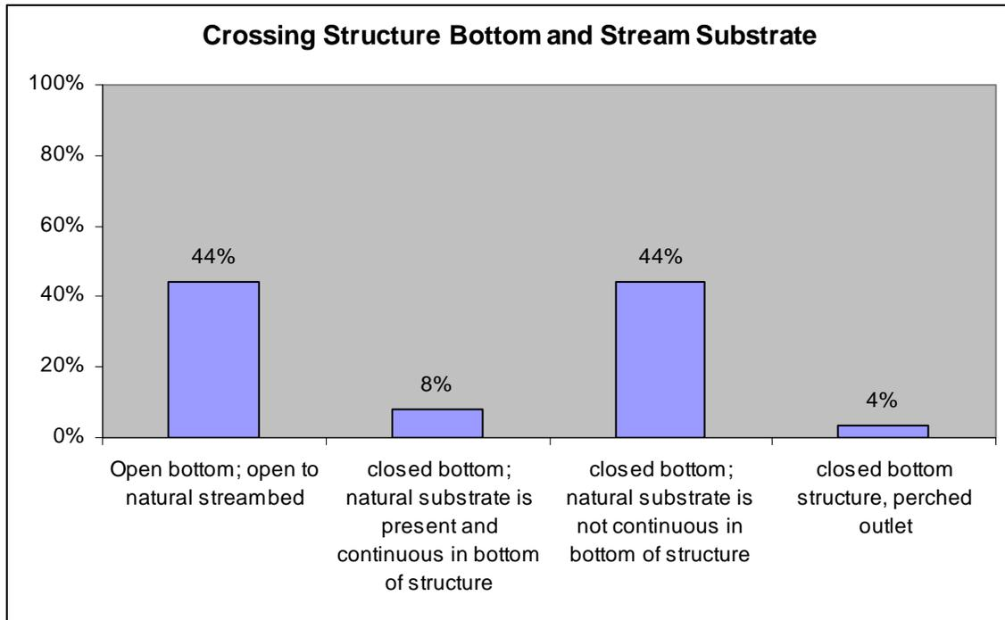
**Figure 16** Presence of substrate in crossing structures. (n=109)
