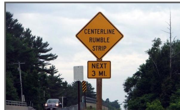
**Centerline rumble strips** are the most common treatment installed on Maine's two lane roads - designed to alert drivers who may be heading for a potentially deadly head on collision, that endangers them and others on the road.
