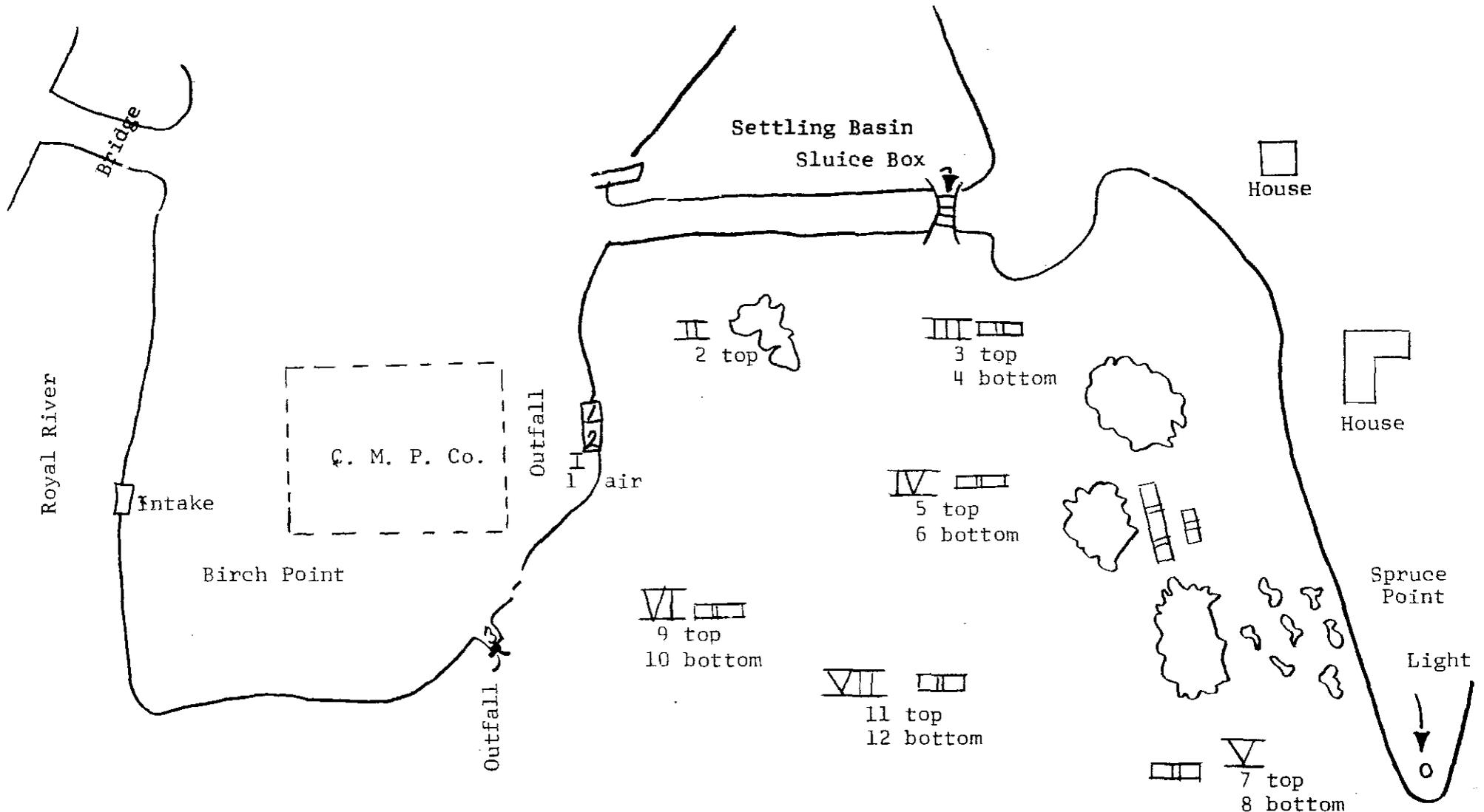
LOCATIONS OF THE SEVEN STATIONS FOR THE THERMOGRAPH WITH TWELVE PROBES. ROMAN NUMERALS DESIGNATE THE STATION NUMBER, WHILE ARABIC NUMBERS DESIGNATE THE PROBE NUMBERS AND WHETHER THE PROBE IS LOCATED AT THE TOP OR BOTTOM OF THE WATER MASS.
