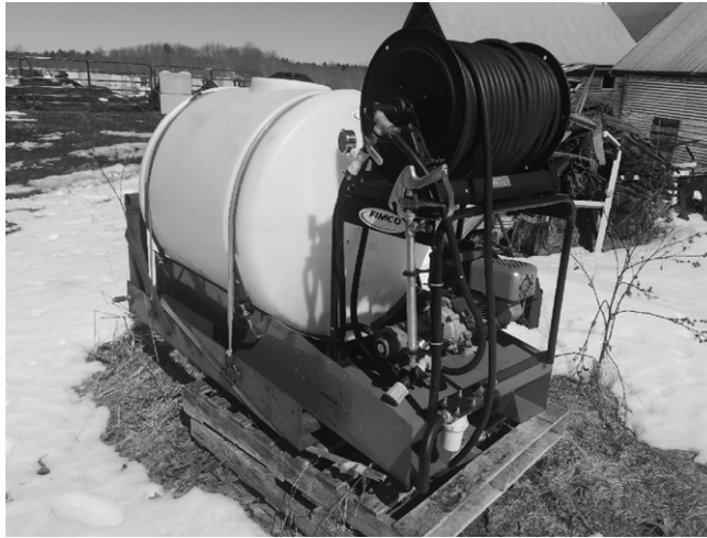
200 Gallon tank used to spray.
