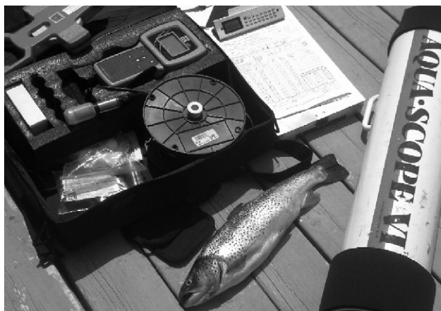
Tools of the trade: WQ Meter, Secchi disk, Aquascope, and nice brown trout caught by fishing at the right depth in the temperature-oxygen profile.
