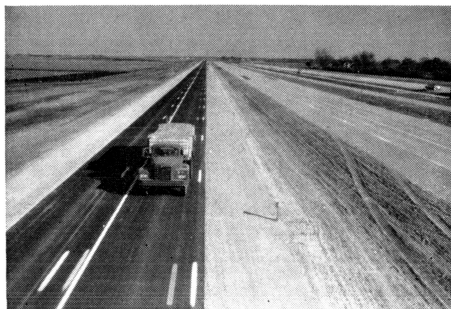
TEST VEHICLE at the AASHO Road Test is shown riding the inner wheel path along a tangent paved with asphaltic concrete. Transverse pattern of truck operation is carefully controlled to simulate pattern found on the highways. Vehicle makes one trip with wheel on outer line, seven with wheel between lines, and two with wheel on inner line.
