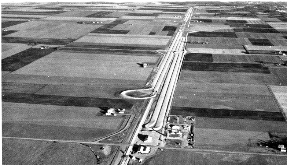
AASHO ROAD TEST site near Ottawa, Illinois, shows one-half of the eight-mile-long research project. Project administration building and maintenance garage are in the foreground. The large loops (left) are two of four main test loops, each with 3.1 miles of two-lane pavement.
