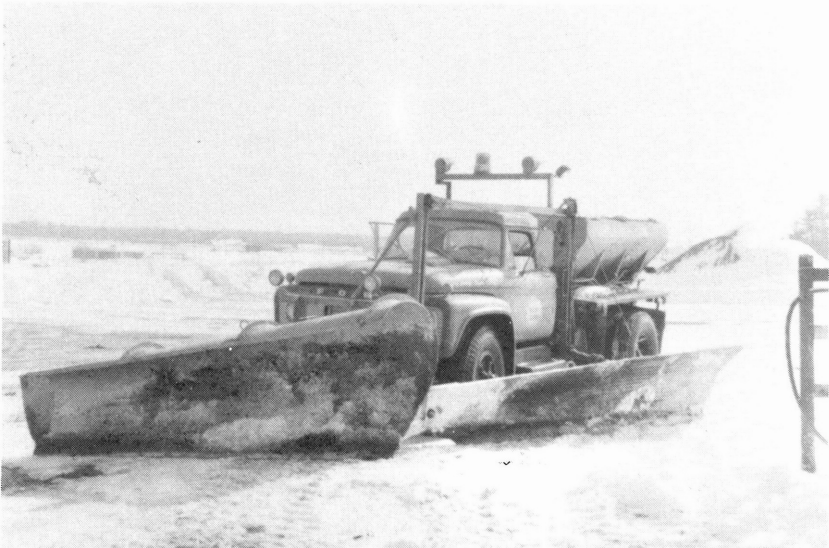
One of our present snow-plowing vehicles equipped for clearing the left lanes.
