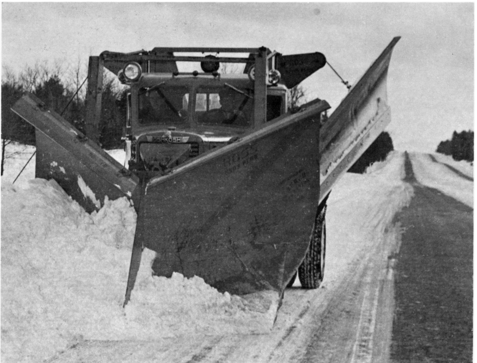
Plowing with one of the original six Oshkosh trucks and a Ross V-plow in January of 1948 . . . our first winter.
