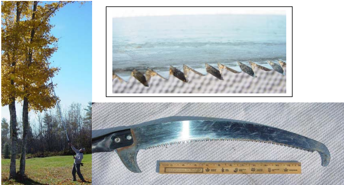
Caption: Silky saws for pruning trees (Insert showing saw teeth). (Photos by SWOAM).
