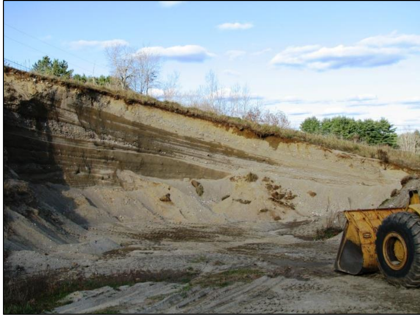
Figure 3.14. Well-stratified sand and gravel in submarine fan exposure near South Jefferson. The parallel relationship between the bedding and ground surface suggests that this fan did not experience any erosion by marine processes after it was deposited.
