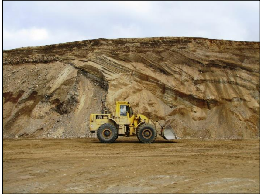
Figure 3.16. The Palmer Hill glacial-marine delta in Whitefield. The upper part of the pit face shows the contact between the horizontal topset beds and inclined foreset beds, which marks the position of sea level when the delta was deposited.
