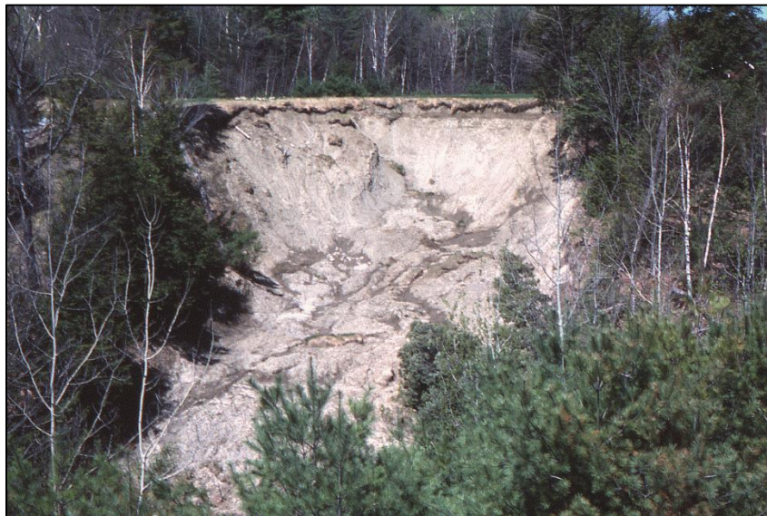
Figure 5.9. Fresh earthflow in the Presumpscot Formation, next to Route 9 in Chelsea. Photo taken in mid 1970s.
