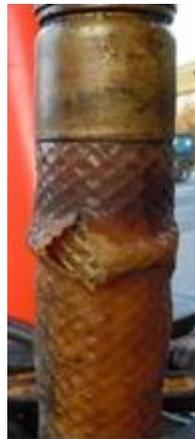
The piping looks as if it may have been bent. It may have grown as it was exposed to moisture, product, and fluctuating temperatures. With nowhere to go, it folded onto itself. Fortunately, only a small amount of product reached the environment and minimal clean-up was required. ♦
