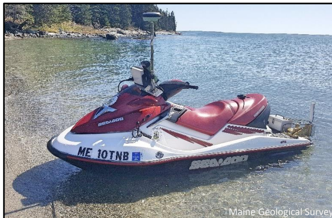
Figures 2a & b. MGS personal watercraft-based bathymetric survey system.
