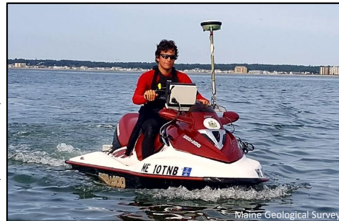
Figures 2a & b. MGS personal watercraft-based bathymetric survey system.
