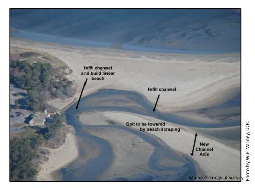
**Figure 7.** Pre-scraping conditions at the Old Morse River channel adjacent to the bath house. Sand would be moved from the spit to infill the channel in front of the bath house, restoring a beach slope, and plugging a constriction in the channel. Closing off the flow would also result in a new and shorter channel in the area marked New Channel Axis.
