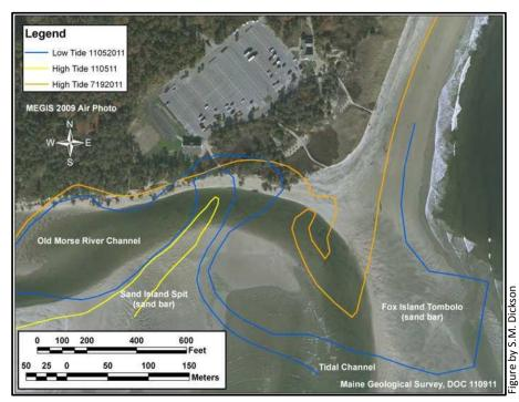
**Figure 5.** The map base is a 2009 air photograph. The blue line is a shoreline survey of the low-tide position of the Old Morse River on November 5, 2011. The orange line is a survey of the July 19, 2011 dune edge (Figure 2). The yellow line is the portion of the sand spit that was above the high tide line on November 5, 2011.
