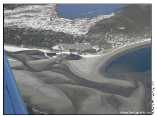
**Figure 11.** Beach scraping infilled the channel and built a beach just seaward of the bath house at the corner of the parking lot at Popham Beach State Park. The new beach face is snow-covered and sloped above the limits of the high tide to provide wave dissipation during winter storms.
