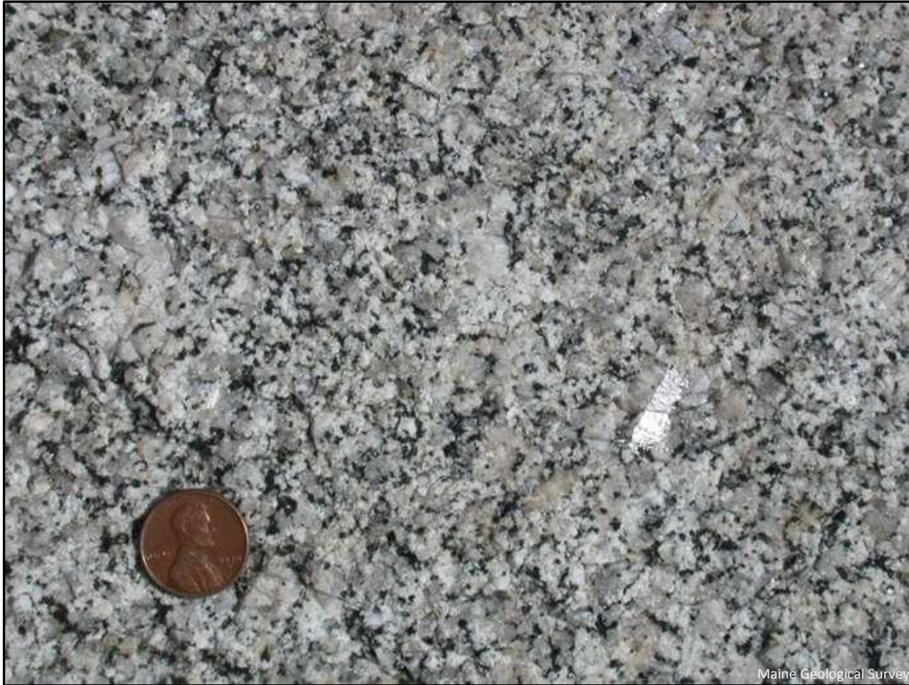
Photo 16. Granodiorite. If sunlight hits a feldspar grain in just the right orientation, you may see a reflection of light like the one in the right-center of this photo.
