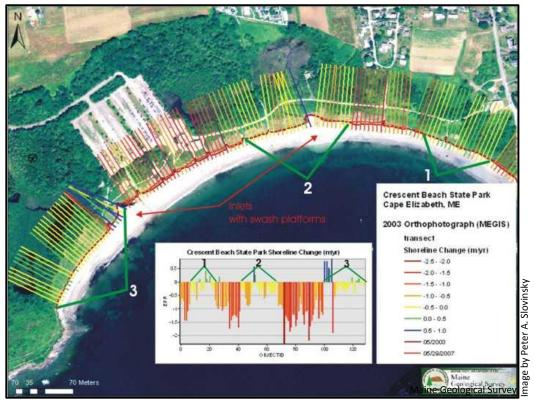
**Figure 8.** Based on shoreline change rates from 2003 to 2007, the Crescent Beach shoreline can be divided into six distinct areas - three that follow highly erosive trends, and three that follow milder and slightly accretive trends (labeled 1, 2, and 3). Base imagery from MEGIS (2003).
