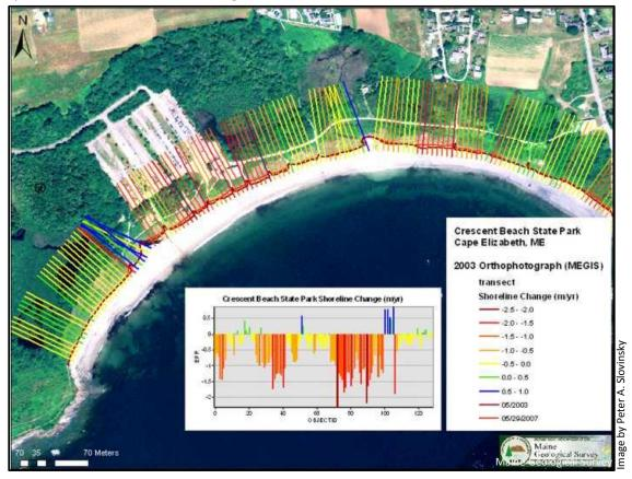
**Figure 3.** Color-coded shoreline change rates along Crescent Beach, calculated from data from 2003 and 2007. Transect numbering in the graph begins on the left at the east end of the beach and progresses right to the west end of the beach. Base imagery from MEGIS (2003).
