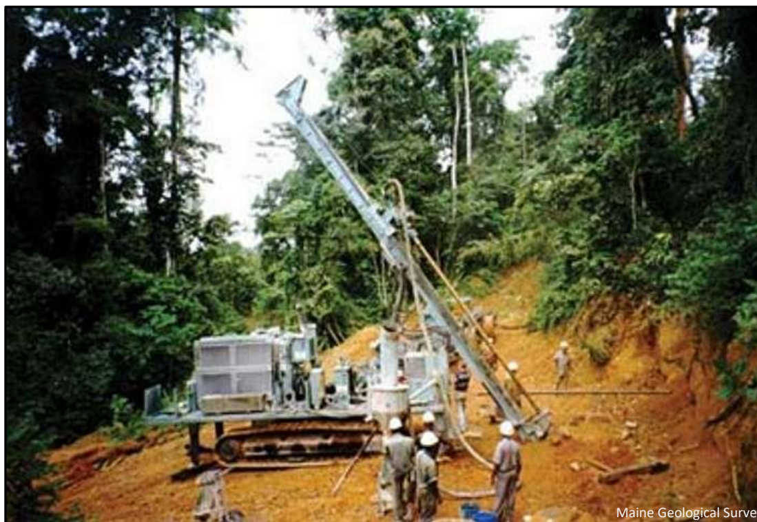
Figure 4. Mineral exploration drill rig drilling a slanted hole into an ore deposit.
