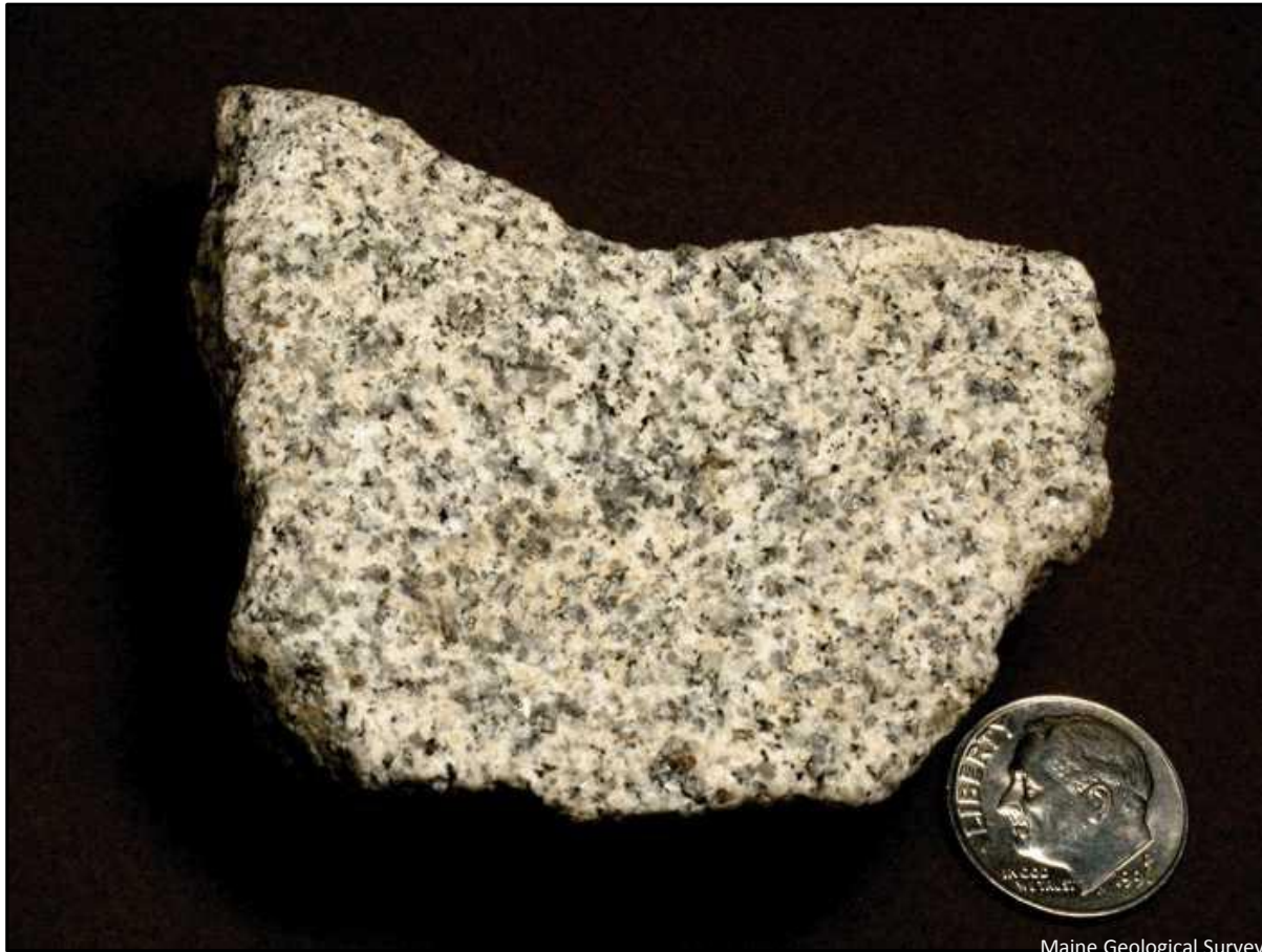
Figure 4. This is a close-up of the granite, showing its equigranular texture. The gray minerals are quartz which makes up about 40-50% of the rock. The white mineral is feldspar which makes up another 40-50%. Biotite, the black flakes, and muscovite which does not show well in the photograph, make up 5-10% of the rock. Minor amounts of other minerals also occur in this rock.
